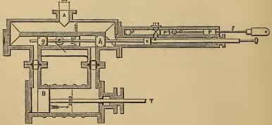
A, the inlet-pipe; a value o serves to regulate the speed of the engine, that is, the expenditure of water. This expedient is serviceable where there is an excess of fall, but it is bad in principle,
